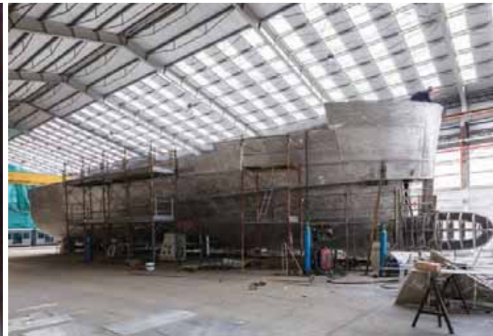
Construction phases of the Aluminum Superyacht.
