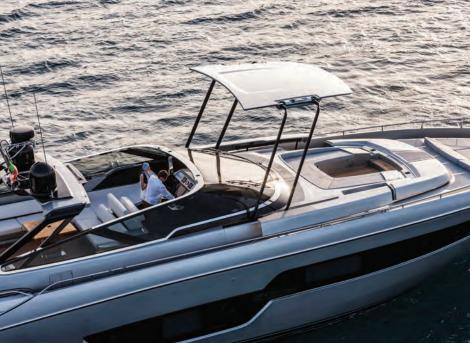
The hard top has been perfectly integrated in both the deckhouse shape and the windshield and roll bar profiles. When it is stored forward, it is kept in place by its own arms, securely connected to the main body.
